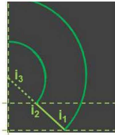
Draw two arcs, centred at i_3 with radius i_1 and i_2
