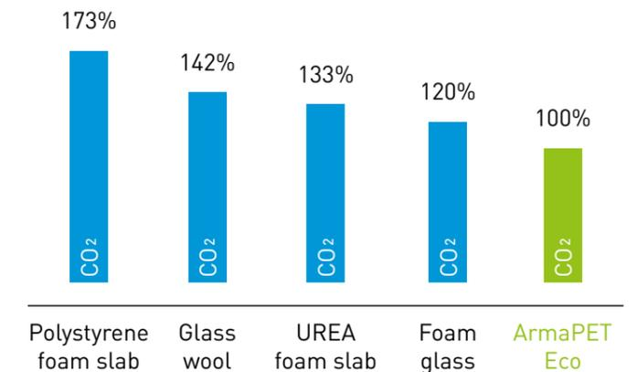
CO<sub>2</sub> emissions of ArmaPET Eco in comparison to competitive materials. ArmaPET Eco = 100% reference
