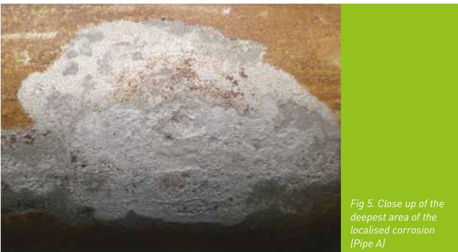
*Fig 5. Close up of the deepest area of the localised corrosion (Pipe A)*
