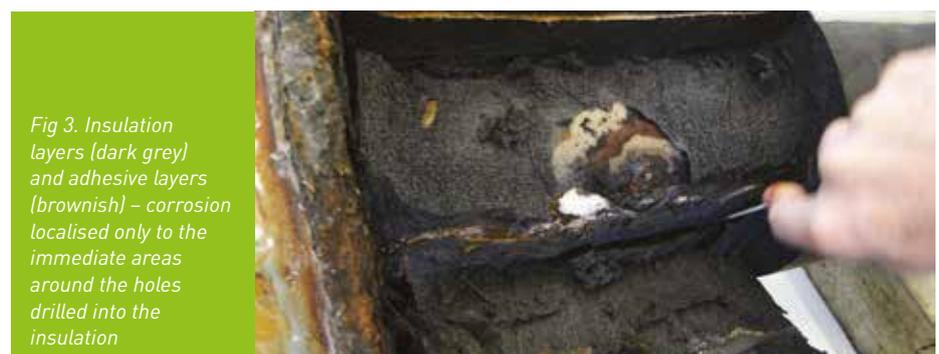
It is important to note that it is the heating of the adhesive used by Armacell (from the 80°C of the water in the pipe) that has caused the general brown discoloration of the pipe surface – it is not the result of corrosion.
