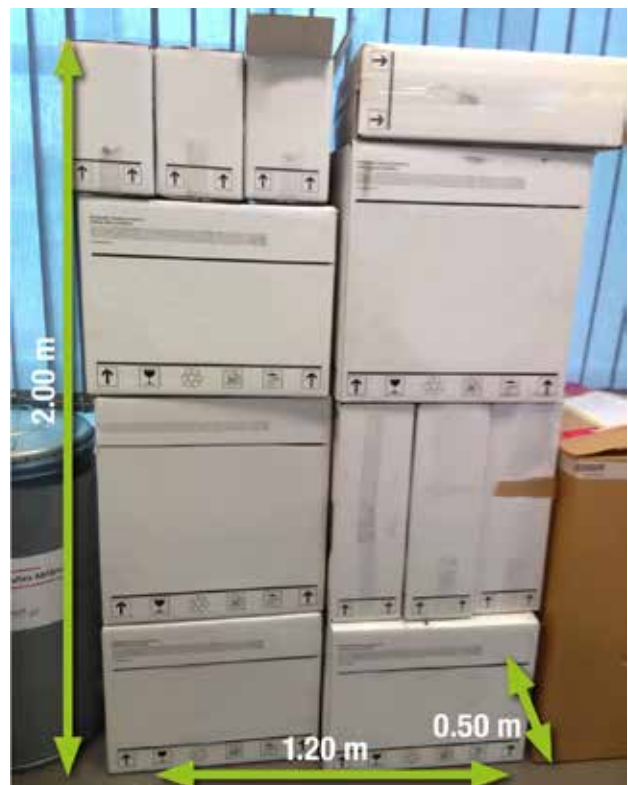
Not really space-saving: when using cellular glass enough storage space must be provided on the building site
