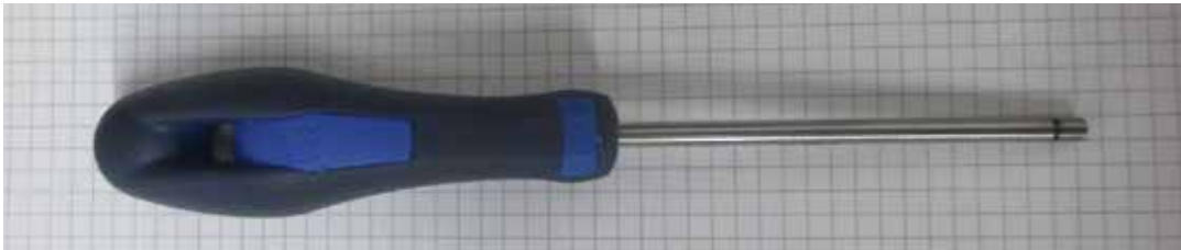
Figure 5: Tool to create punch holes in insulation systems.
