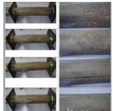
Figure 13: Pipe surface of Sample C, glass fibre, after 65 days.
