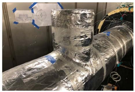
Figure 9: First insulation layer
